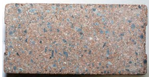
Permaflow Bond 80 Tan Cut Face Dimensions 200 x 100 x 80mm 50 Pavers per Square Meter Abrasion Index \leq 12 gram Strength 45Mpa Weight 4.5kg
