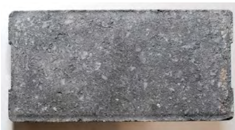
Permaflow Bond 80 Charcoal Dimensions 200 x 100 x 80mm 50 Pavers per Square Meter Abrasion Index \leq 12 gram Strength 45Mpa Weight 4.5kg
