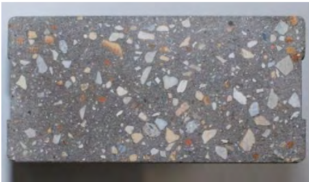
Permaflow Bond 80 TMS Brown Cut- Face Dimensions 200 x 100 x 80mm 50 Pavers per Square Meter Abrasion Index \leq 12 gram Strength 45Mpa Weight 4.5kg
