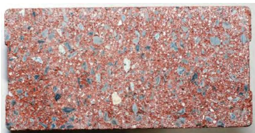
Permaflow Bond 80 Terracotta Cut Face Dimensions 200 x 100 x 80mm 50 Pavers per Square Meter Abrasion Index \leq 12 gram Strength 45Mpa Weight 4.5kg
