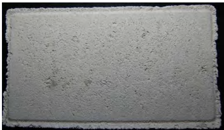
Permaflow Bond 80 White Dimensions 200 x 100 x 80mm 50 Pavers per Square Meter Abrasion Index \leq 12 gram Strength 45Mpa Weight 4.5kg
