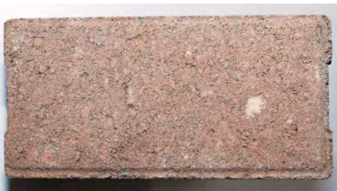
Permaflow Bond 80 Tan Dimensions 200 x 100 x 80mm 50 Pavers per Square Meter Abrasion Index \leq 12 gram Strength 45Mpa Weight 4.5kg
